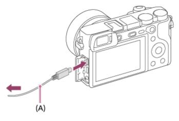
If you connect the product to your computer using the micro USB cable when [USB Power Supply] is set to [On], power is supplied from your computer. (Default setting: [On])
