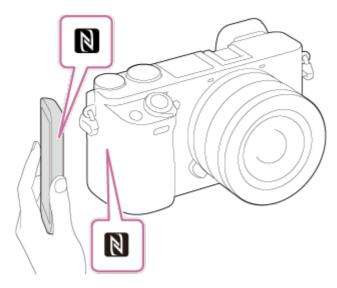
The product and the smartphone are connected, and PlayMemories Mobile automatically launches on the smartphone, and then the displayed image is sent to the smartphone.
