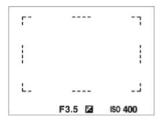
When you use a zoom function other than the optical zoom, the [Focus Area] setting is disabled and the focus area frame is shown by the dotted line. The AF operates with priority on and around the center area.
