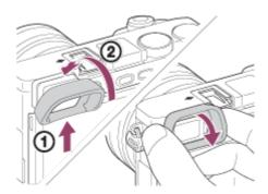
• Remove the eyepiece cup when you attach an accessory (sold separately) to the Multi Interface Shoe.
