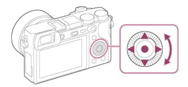
You can select setting items by turning or pressing the top/bottom/right/left side of the control wheel. Your selection is determined when you press on the center of the control wheel.
