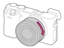
• Be sure to hold the lens straight when attaching it.
