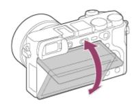
You may not be able to adjust the monitor angle depending on the type of a tripod you use. In such a case, release the tripod screw once to adjust the monitor angle.
