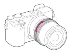
When you rotate the focus ring, the focus distance is displayed on the screen.
