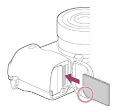
• Ensure that the notched corner is facing in the correct direction.
