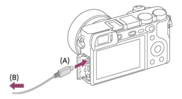
**A:** To the Multi/Micro USB Terminal **B:** To the USB jack of the computer
