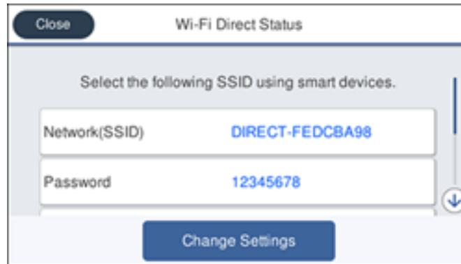
6. Use your computer or wireless device to select the Wi-Fi network name (SSID) displayed on the LCD screen, then enter the password shown.
