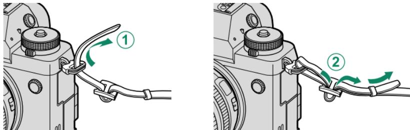
**!** To avoid dropping the camera, be sure the strap is correctly secured.
