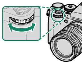
**FUNCTION/DIAL SETTING** Aperture control defaults to the front command dial, but can be reassigned to the rear command dial using **FUNCTION/DIAL SETTING > COMMAND DIAL SETTING**.
