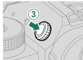
**!** Lift the control before use. Failure to observe this precaution could cause product malfunction.
