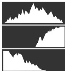
To view separate RGB histograms and a display showing areas of the frame that will be overexposed at current settings superimposed on the view through the lens, press the function button to which **HISTOGRAM** is assigned (📖 295, 321).
