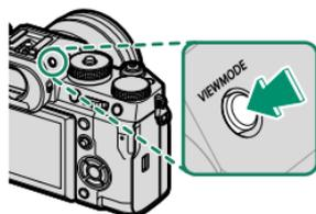
Use **SCREEN SET-UP > VIEW MODE SETTING** in the setup menu to choose a display mode for the EVF and LCD monitor.
