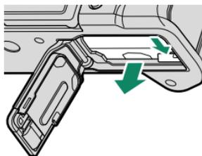
⚠ The battery may become hot when used in high-temperature environments. Observe caution when removing the battery.
