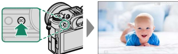
Additional pictures can be viewed by pressing the selector left or right or rotating the front command dial. Press the selector or rotate the dial right to view pictures in the order recorded, left to view pictures in reverse order. Keep the selector pressed to scroll rapidly to the desired frame.
