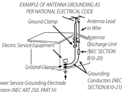
**Power Lines:** An outside antenna system should not be located in the vicinity of overhead power lines or other electric light or power circuits, or where it can fall into such power lines or circuits. When installing an outside antenna system, extreme care should be taken to keep from touching such power lines or circuits as contact with them might be fatal.
