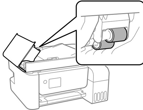
**Caution:** Using a dry cloth may damage the surface of the rollers. Let the rollers dry before using the ADF.
