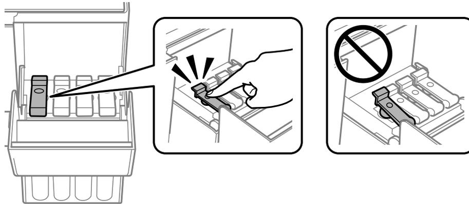
**Note:** Do not leave the ink bottle inserted. The bottle may be damaged or ink may leak. If any ink remains in the bottle, replace the bottle cap and tighten it. Store the bottle upright for later use.
