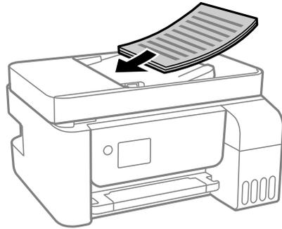
**Note:** Do not load originals above the arrow mark on the ADF edge guide.
