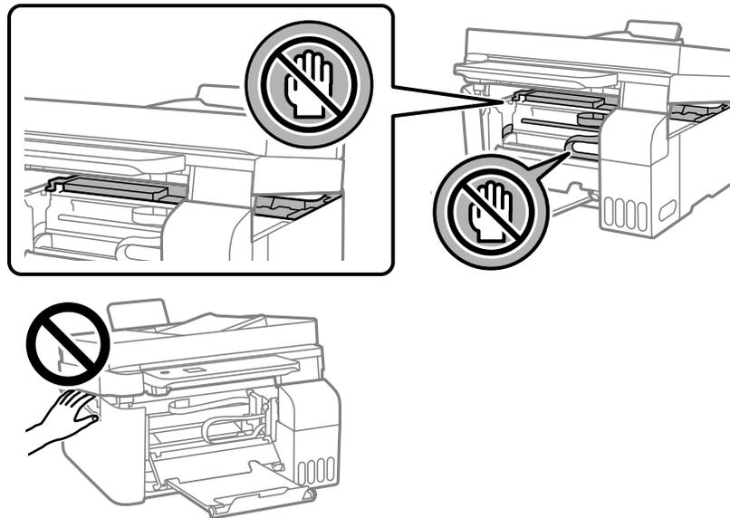
7. Lift the scanner unit up slightly and lower it. When the scanner unit catches, lift it up again and lower it completely.
