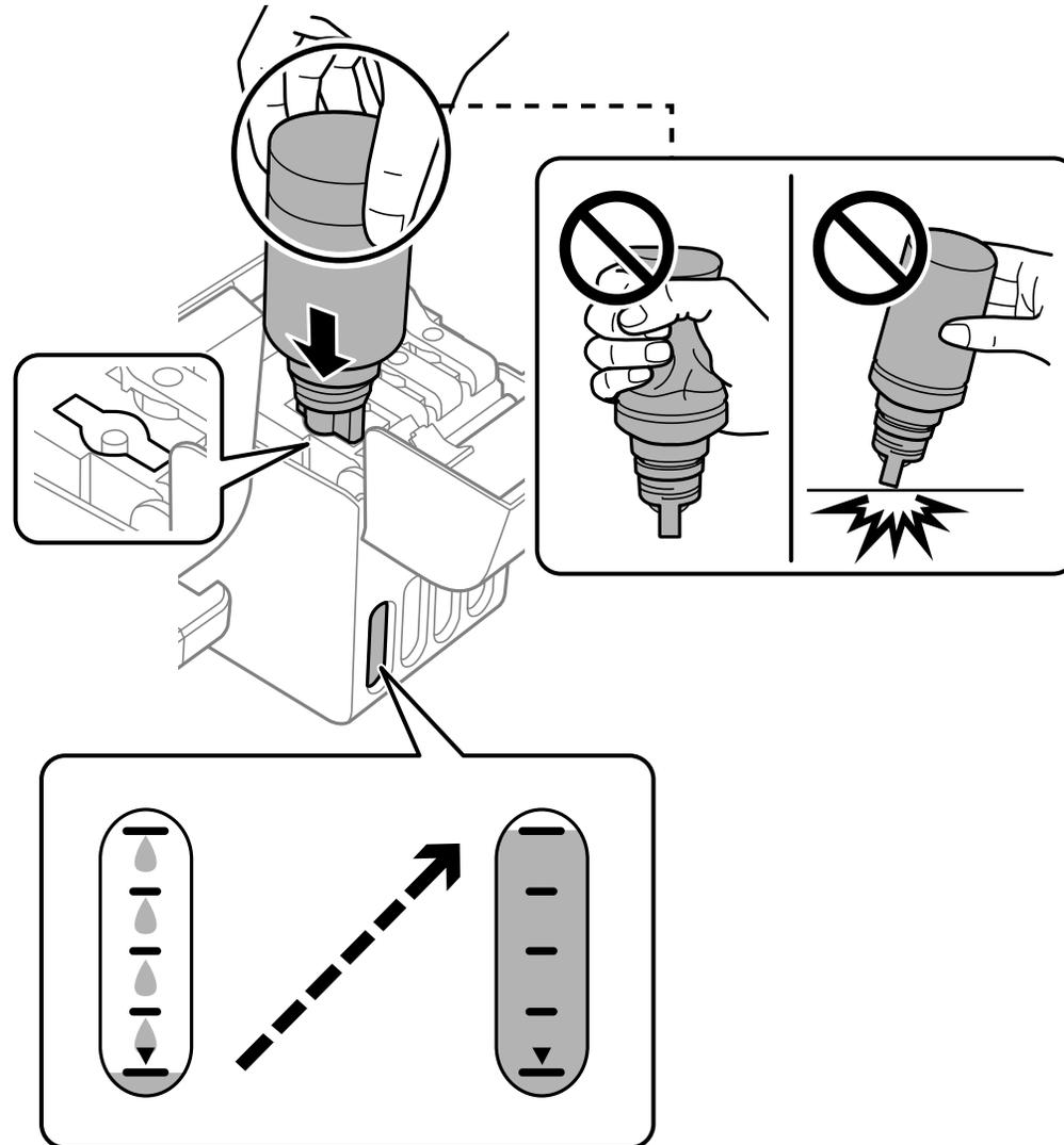
**Note:** If ink does not flow from the bottle, lift and reinsert the bottle. If the ink has reached the upper line of the tank, do not remove and reinsert the bottle or ink may leak.
