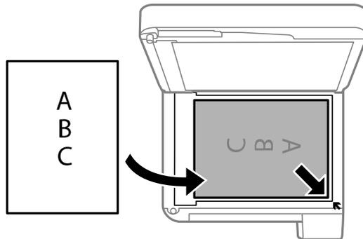
**Note:** If you are using Epson ScanSmart to scan multiple photos at once, just make sure they are at least 0.2 inch (4.5 mm) away from the edge of the scanner glass and at least 0.8 inch (20 mm) away from each other.
