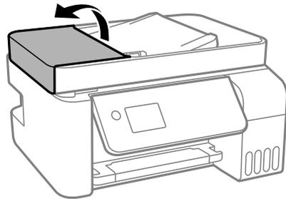
10. Use a soft, moistened, lint-free cloth (microfiber is recommended) to clean the rollers and the interior of the ADF.
