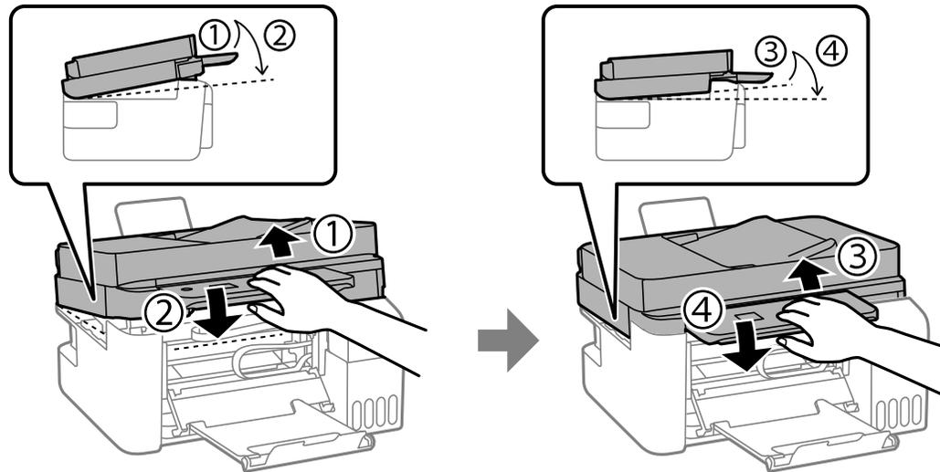
**Note:** The scanner unit must be closed completely before it can be opened again.
