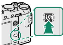
Indicators for the EVF and LCD must be selected separately. To choose the EVF display, place your eye to the viewfinder while using the **DISP/BACK** button.
