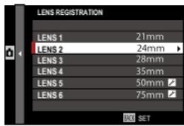
For other lenses, select **LENS 5** or **LENS 6** and use the focus stick (focus lever) to enter the focal length.
