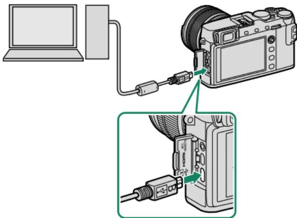
**!** The USB cable must be no more than 1.5 m (4.9 ft.) long and be suitable for data transfer.
