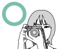
To prevent pictures that are out of focus or too dark (underexposed), keep your fingers and other objects away from the lens and AF-assist illuminator.
