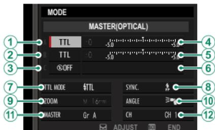
The master and remote units can be placed in up to three groups (A, B, and C) and flash mode and flash level adjusted separately for each group. Four channels are available for communication between the units; separate channels can be used for different flash systems or to prevent interference when multiple systems are operating in close proximity.
