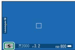
**!** If the correct exposure cannot be achieved at the selected shutter speed, aperture will be displayed in red. If the subject is outside the metering range of the camera, the aperture display will show “— —”.
