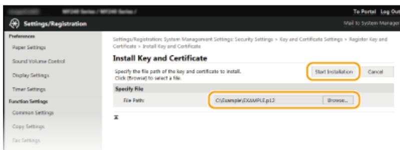
⇒ The key pair or CA certificate is installed in the machine.
