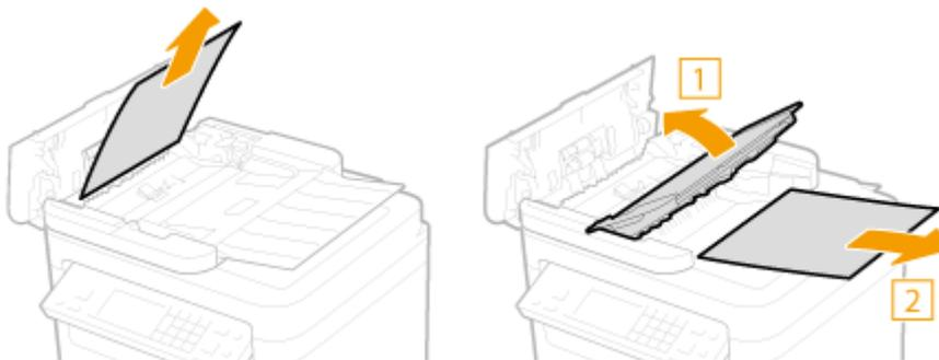
**2 Remove the jammed document from the inner cover inside the feeder.**
