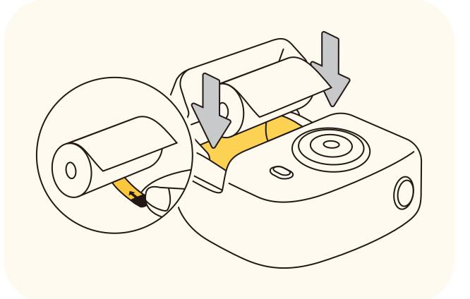
4 Pull the paper roll out of the outlet and close Front Cover
