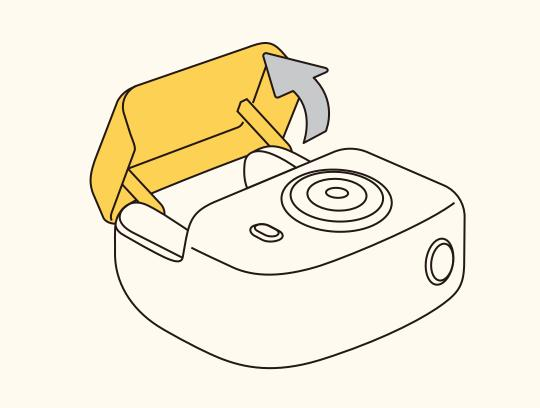
3 Pull the paper out of the slot and close Front Cover
