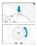
Press a button such as < MODE > or < M-Fn >, then turn the <  $\bigcirc$  > dial.
