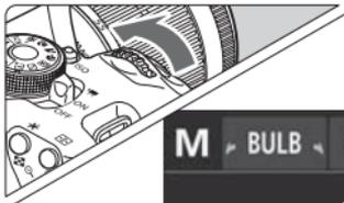
A bulb exposure keeps the shutter open for as long as you hold down the shutter button. It can be used to photograph fireworks and other subjects requiring long exposures. In step 3 on the preceding page, turn the <☀> dial to the left to set <BULB>. The elapsed exposure time will be displayed on the LCD monitor.
