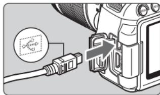
**3** Connect the camera to the printer.
