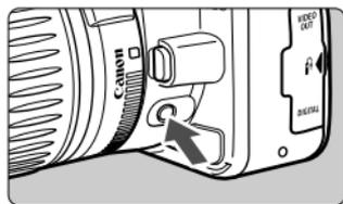
Press the depth-of-field preview button to stop down to the current aperture setting. The diaphragm in the lens will close to the current aperture and you can check the depth of field (range of acceptable focus) through the viewfinder.
