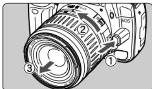
**While pressing the lens release button, turn the lens as shown by the arrow.**
