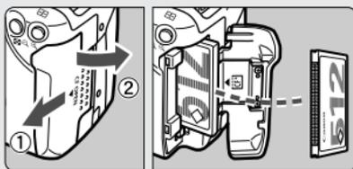
**Open the CF card slot cover and insert a CF card.** (p.26)
