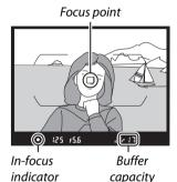
While the shutter-release button is pressed halfway, the number of exposures that can be stored in the memory buffer ("#" \( \sigma \) 58) will be displayed in the
