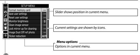
If a ? icon is displayed at the bottom left corner of the monitor, help can be displayed by pressing the  $\textcircled{?}/\multimap$  (WB) button. A description of the currently selected option or menu will be displayed while the button is pressed. Press  $\blacktriangle$  or  $\blacktriangledown$  to scroll through the display.
