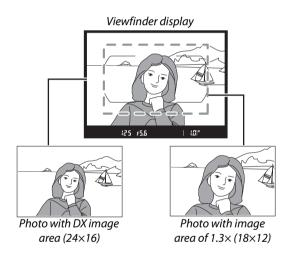
Image area can be set using the **Image area** option in the shooting menu or by pressing a control and rotating a command dial ( $\square$  65).
