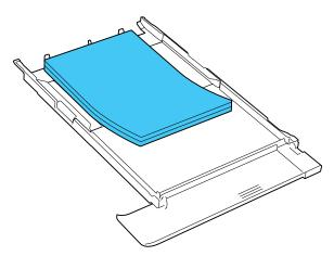
• Insert up to 10 envelopes, printable side down and flap edge left, as shown.
