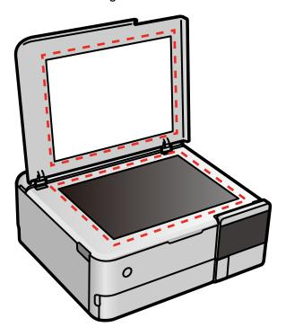
**Caution:** Do not spray glass cleaner directly on the glass and wipe off all remaining liquid. Do not press the glass surface with any force.
