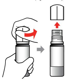
**Caution:** Do not shake or squeeze the ink bottle. Do not touch the top of the bottle after its cap is removed.
