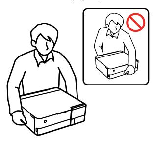
• Avoid tilting the product, placing it vertically, or turning it upside down; otherwise ink may leak. When storing or transporting the printer, place it in a plastic bag and fold it closed.
