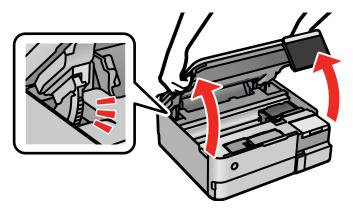
3. Open the ink tank cover, then open the cap for the ink tank you are going to fill.
