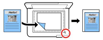
**Note:** The edges of your original may be cropped by 0.06 inch (1.5 mm) from the edge of the scanner glass. Manually position your original away from the edges to prevent cropping.
