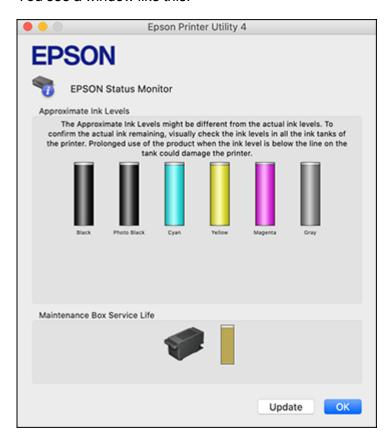
3. Refill any ink tank or replace the maintenance box as needed.
