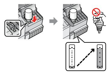
**Note:** Refer to the color-coded sticker on the ink tank unit to identify the color of each tank. Do not force the bottles into position; they are keyed for each color.
