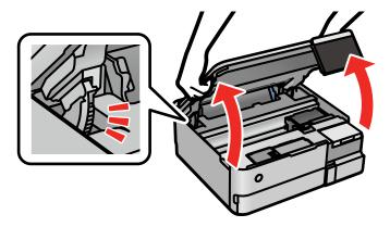
8. Make sure the print head is in the home position on the right and move the transportation lock to the transport position.
