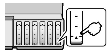
**Note:** The product has a low ink alert system. The accuracy of this system depends on the user refilling the ink tanks correctly. The product cannot directly measure the ink levels in the tanks; instead it estimates the amount of ink remaining by internally monitoring ink usage. The low ink alert system may generate inaccurate messages if the ink tanks are not refilled according to these instructions.
