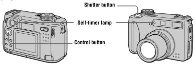
Clear the menu (page 41), then press the control button  $\nabla$  (§). The § (self-timer) indicator appears on the LCD screen, and about 10 seconds after you press the shutter button, the subject is recorded. The self-timer lamp flashes and the beep sounds after you press the shutter button until the shutter is released. To cancel the self-timer recording, press the control button  $\nabla$  (§) again.
