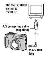
Connect the A/V connecting cable to the A/V OUT jack of your camera and to the audio/video input jacks of the TV.
