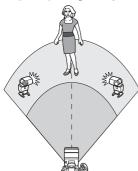
Effective when you need a large flash output. All the slave units will fire at the same output and be controlled to obtain a standard exposure.
