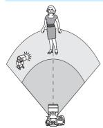
This is fully automatic wireless flash shooting with <u>one external Speedlite and</u> the built-in flash.
