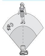
This shows the most basic setup for fully-automatic wireless flash shooting with one external Speedlite.
