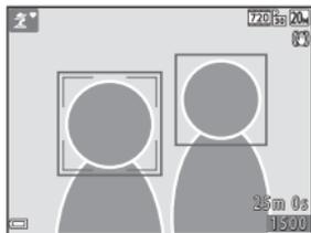
If the camera detects more than one face, a double border is displayed around the face that the camera focuses on, and single borders are displayed around the other faces.
