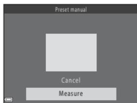
**4** Frame the white or gray reference object in the measuring window, and press the **OK** button to measure the value.
