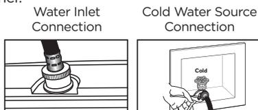
**!** The hose connected to the COLD water source must be connected to the COLD water supply intake.
