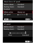
You can set the Movie Servo AF's AF speed and its operation conditions. This function is settable when [Movie Servo AF] is set to [Enable] and [AF method] is set to [FlexiZone - Single]. Additionally, the function is only enabled when using a lens compatible with slow focus transition during movie shooting\*.
