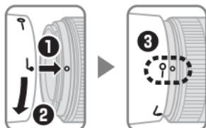
*Align the lens hood lock mark (—○) with the lens hood mounting mark (●) on the lens (❸).*
