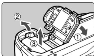
**2** Open the cover and remove the battery.
