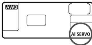
**While you press the shutter button halfway, the camera focuses continuously.**
