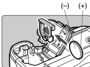
**4** Replace the battery in the battery holder.
