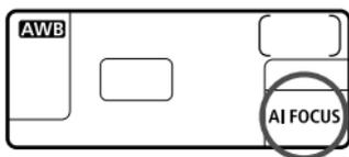
AI Focus AF switches the AF mode from One-Shot AF to AI Servo AF automatically if the still subject starts moving.
