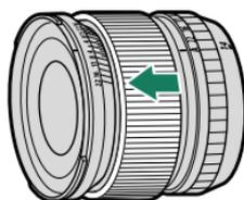
For manual focus, slide the focus ring to the back and rotate it while checking the results in the camera display. The focus distance and depth-of-field indicators can be used to assist manual focus.
