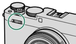
The roles assigned to the front command dial during shooting can be chosen using **FUNCTION/SETTING > COMMAND DIAL SETTING** (📖 226). At default settings, the dial can be used in the following three roles:
