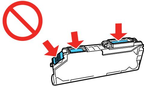
6. Remove the cap from the cartridge and save the cap so you can recap ink cartridges before storing or disposing of them.
