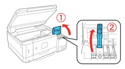
Unpack the ink bottle that matches the open ink tank. Hold the ink bottle upright and slowly turn the bottle cap to remove it.
