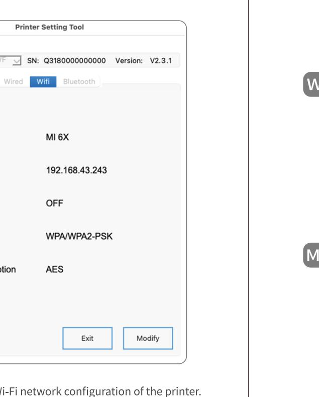
**English** Enter the Wi-Fi password. Complete the Wi-Fi network configuration of the printer.
