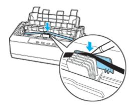
g Turn the ribbon-tightening knob in the direction of the arrow to help feed the ribbon into place; it should not be twisted or creased.
