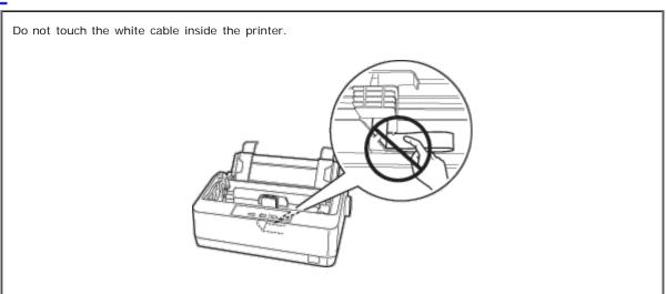
8 Use a pointed object, such as a ball point pen, to guide the ribbon between the print head and ribbon guide.
