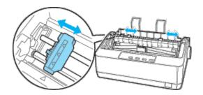
Make sure your paper has a clean, straight leading edge. Open the sprocket covers. Fit the first holes of the paper over the sprocket pins and then close the sprocket covers. Slide the right sprocket unit to remove any slack in the paper and lock it in place. Now the paper is in the paper-park position.
