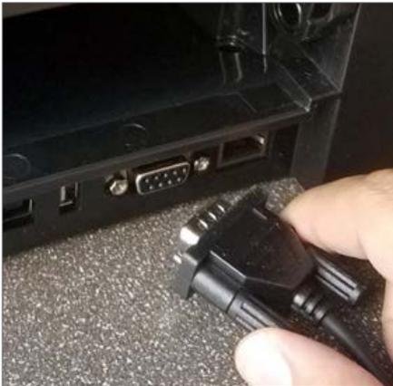
5. Connect the Striker Keypad to the printer
