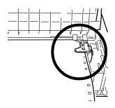
10 Adjust the left tractor until the holes in the paper are centered on the pins then lock the lever and close the left tractor cover.
