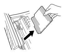
3 Remove the shipping restraint from the pull-up roller assembly (1).
