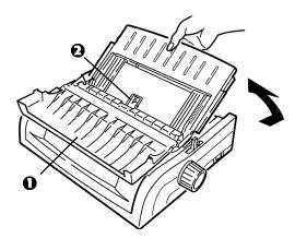
**4** Adjust the paper feed guides (1) for the width of the paper, then place a sheet of paper in the separator. The paper will feed into the printer.
