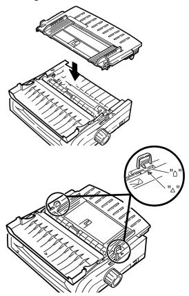
**10** Place the wire guide (1) in the sheet guide on the pull-up roller assembly.
