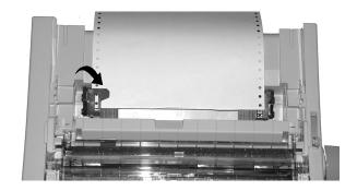
**8** Adjust the position of the right tractor to center the holes in the paper on the pins. Then, close its tractor cover and push back the lock lever. Do not stretch the paper.
