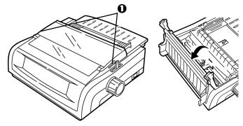
2 Remove the printhead shipping restraint.
