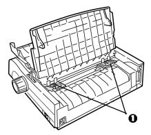
6 Open the lock levers (1) and move the right tractor (as viewed from the back of the printer) to the reference mark
