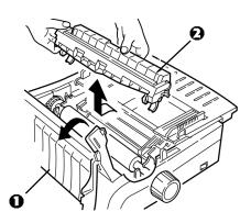
5 Lift the sheet guide (1) and reload paper. Make sure you lock the tractor covers.
