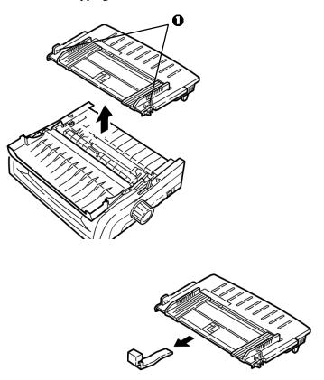
**5** Reinstall the sheet guide: insert the clips on either side of the separator into the notches marked with a triangle, then press down to secure the separator in place.
