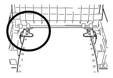
11 Lower the sheet guide and slide it toward the front of the printer until the marks align.
