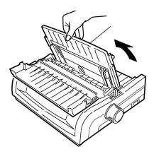
**5** From the back of the printer, locate the tractors (1).
