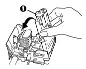
**4** Turn the take-up knob (1) in the direction of the molded-in arrow to take up any ribbon slack.
