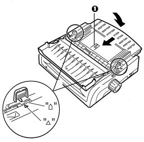
**12** Place the wire guide ("1" in the illustration for the step above) in the sheet guide on the pull-up roller assembly.
