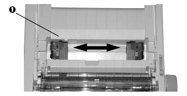
7 Open the tractor covers and place continuous forms paper on the first two pins of either tractor, then close the *left* tractor cover.
