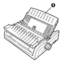
**3** Pivot the wire feed guide into the sheet guide.
