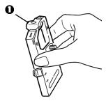
Remove the ribbon cartridge and check the ribbon shield.
