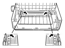
**8** Place continuous forms paper on the first two pins of either tractor.
