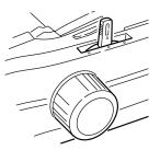
**3** Open the acoustic cover (1) and raise the sheet guide to the single-sheet position. Pivot the wire feed guide (2) up into the sheet guide.
