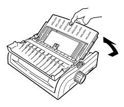
4 Pivot the sheet guide forward and gently rest it against the roller assembly.
