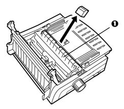
**4** Use the tabs (1) to lift and remove the sheet guide, then remove the shipping restraint.
