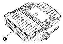
**3** Grasp the tabs and lift off the sheet guide.
