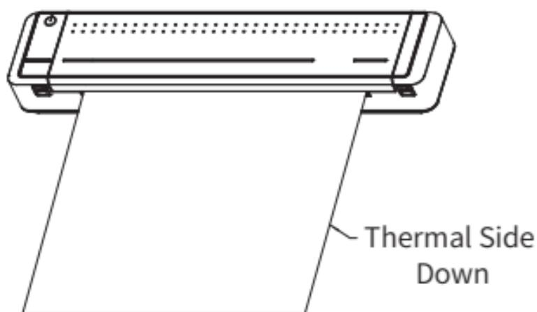
**Note:** If the buzzer sounds once when paper feeding stops, it shows that the paper is loaded successfully. If the buzzer keeps beeping and the red LED is flashing, please open the cover and reload the paper.
