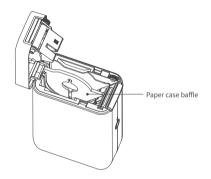
3. Requirements for installation of paper case baffle (the baffle has been installed before delivery, and can be used directly for 15mm backing paper labels, but should be removed for 27mm backing paper labels).
