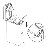
4. Installation of consumables: Insert the roll of paper on the right, with the printing surface facing the switch.
