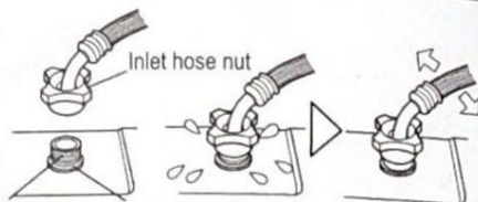
Inlet valve connector Water absorption cushion
