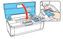
6 Press the ∆ ink button to begin priming the ink. This takes about 3 minutes. Do not turn off the printer, load paper, or open any covers until the process is complete.
