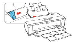
4 Load paper printable side up (usually the whiter, brighter, or glossy side), against the right edge of the sheet feeder, and behind the tab. Then squeeze the left edge guide and slide it against the left edge of the paper, but not too tightly.
