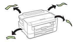
2 Open the printer cover and remove all protective materials from inside the product.
