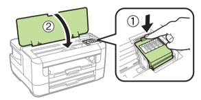
7 The printer starts charging the ink. Ink charging takes approximately 6 minutes. When you see a completion message on the printer's LCD screen, charging is complete.
