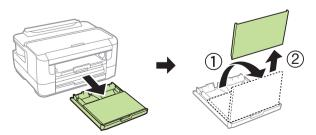
**2** Slide the side edge guides all the way out and set the front edge guide to the paper size you are using.
