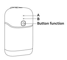
A is a two-color light, with white representing "1 hour" and green representing "2 hours". B is a white lamp with UV function.
