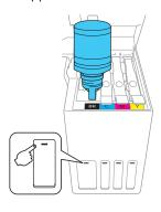
**Note:** If ink does not flow from the bottle, lift and reinsert the bottle.
