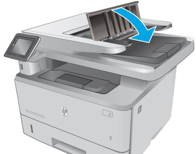
7. Open the scanner lid. If paper is jammed in the scanner lid, gently pull it out, and then close the scanner lid.
