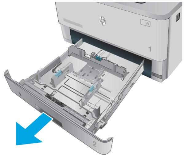
2. Adjust the paper-width guides by squeezing the adjustment latch on the left guide and sliding the guides to the size of the paper being used.
