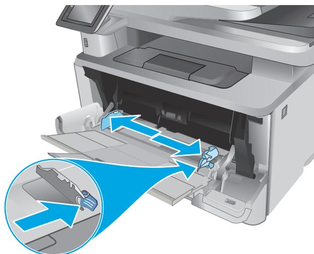
5. Load the paper into the tray. Make sure that the paper fits under the tabs and below the maximum-height indicators.
