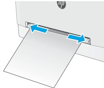
2. Place the top edge of the sheet at the opening, and then adjust the side guides so that they lightly touch the sheet, but do not bend it.
