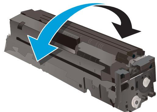
7. Install the new toner cartridge. Make sure that the color chip on the cartridge matches the color chip on the drawer.
