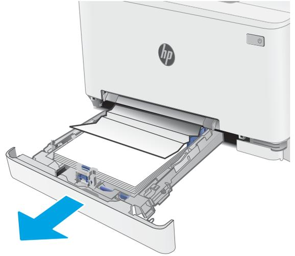
2. Remove any jammed or damaged sheets of paper.
