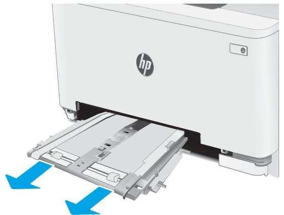
4. Remove any jammed or damaged sheets of paper.
