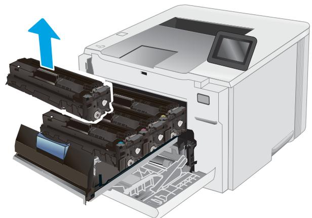
4. Remove the new toner cartridge package from the box, and then pull the release tab on the packaging.
