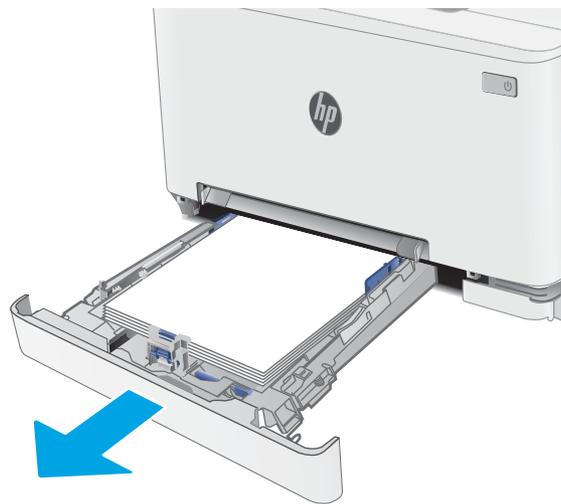
2. Push down on the single-sheet priority feed slot, and then pull out the feed slot tray.
