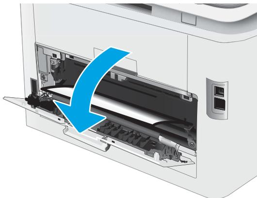
2. If paper is visible in the output bin, grasp the leading edge and remove it. Use both hands to remove jammed paper to avoid tearing the paper.
