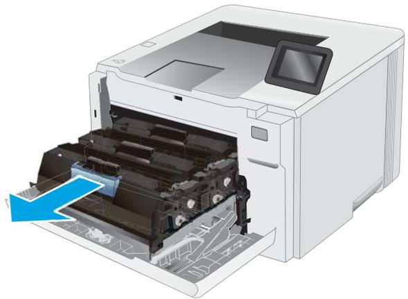
3. Grasp the handle on the toner cartridge, and then pull the toner cartridge straight up to remove it.
