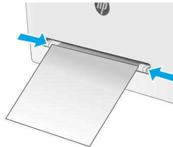
3. Insert the single sheet into the slot and hold it. The printer will pull the sheet partially into the paper path. For information about how to orient the paper, see [Tray 1 paper orientation on page 18](#).
