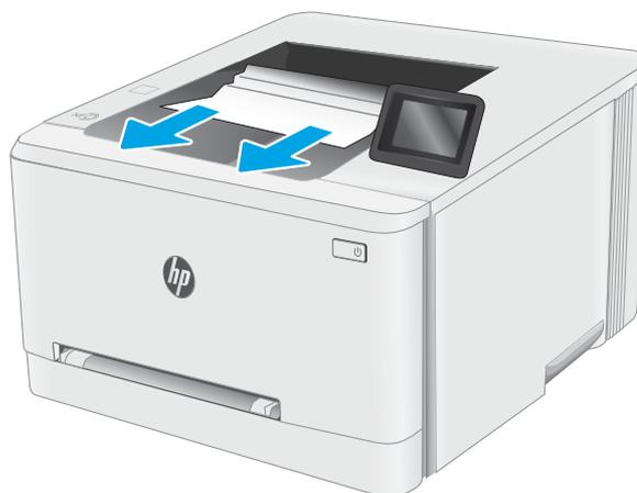
3. Gently remove any jammed paper from the rollers in the rear door area.
