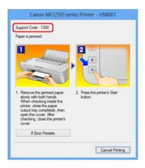
For details on how to remove the jammed paper, refer to <u>Support Code List (When Paper Is</u> Jammed).
