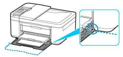
Open the paper output tray, then press the printer's **OK** button.
