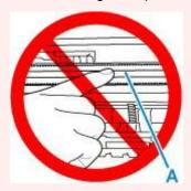
If you soil or scratch this part by touching it with paper or your hand, it could damage the printer.
