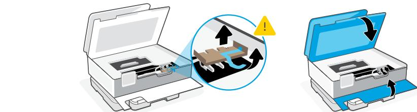
EN Remove all packaging and tape. Open the front door and cartridge access door. Remove cardboard. Make sure to close the doors.
