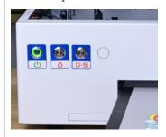
1.5 The printer is ready once the power light stops flashing
