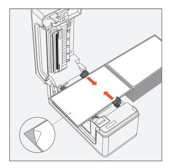
Please place the labels with the tear-off side facing up as shown in the picture above.
