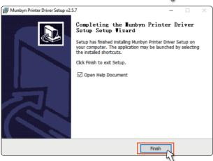
After the driver installation is complete, the printer will appear in your printer list, If Munbyn does not appear on your computer, please restart the printer and computer.
