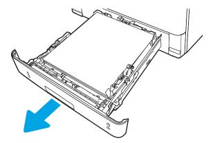
2. Remove the paper from the tray, and discard any damaged paper.
