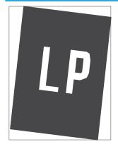
The image is not centered, or is skewed on the page. The defect occurs when the paper is not positioned properly as it is pulled from the tray and moves through the paper path.
