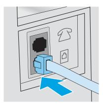
4. Connect the answering machine telephone cable to the telephone line out port on the rear of the printer.
