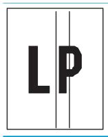
Dark vertical lines which occur down the length of the page. The defect might occur anywhere on the page, in areas of fill or in sections with no printed content.
