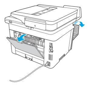
10. If jammed paper is visible, remove any jammed paper from the rear door area.
