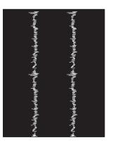
Table 9-8 Fixing/fuser defects on page 157
