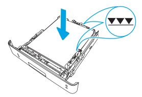
5. Slide the tray completely into the printer.
