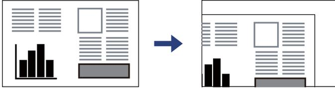
3. Place the original face-down and slide it to the corner mark.
