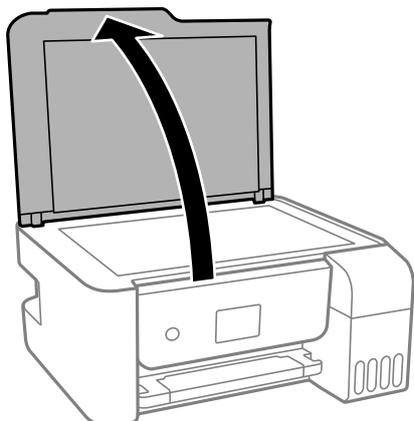
2. Use a soft, dry, clean cloth to clean the surface of the scanner glass.
