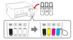
**Caution:** After setup, periodically inspect the ink levels to ensure they do not fall below the ▼ lower lines. Prolonged use when any level is lower than the line could damage the product. See the online *User's Guide* for refilling instructions.
