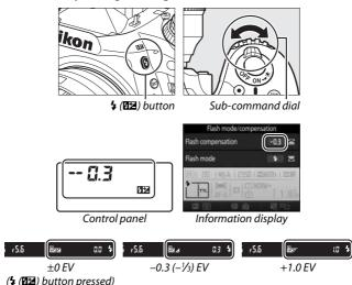
At values other than  $\pm 0.0$ , a  $\square$  icon will be displayed in the control panel and viewfinder after you release the  $\frac{1}{2}$  ( $\square$ ) button. The current value for flash compensation can be confirmed by pressing the  $\frac{1}{2}$  ( $\square$ ) button.
