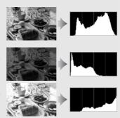
Increasing exposure compensation shifts the distribution of tones to the right, while decreasing exposure compensation shifts the distribution to the left. Histograms can provide a rough idea of overall exposure when bright ambient lighting makes it difficult to see photographs in the monitor.
