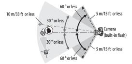
Wireless remote sensors on flash units should face camera.
