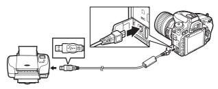
When the camera and printer are turned on, a welcome screen will be displayed in the monitor, followed by a PictBridge playback display.
