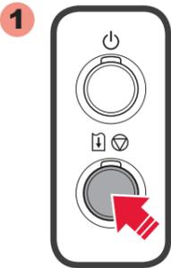
**EN** If the **Alarm** lamp flashes orange, press the **RESUME/CANCEL** button, then proceed to 6. Print Head Alignment can also be performed after installation.
