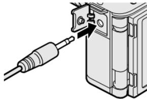
A confirmation dialog will be displayed when a third-party release is connected; press **MENU/OK** and select **REMOTE** for **MOVIE SET-UP > MIC/REMOTE RELEASE.**
