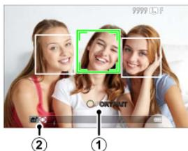
**!** In **SR+** mode, the camera continuously adjusts focus and searches for eyes, increasing the drain on the battery; in addition, the sound of the camera focusing may be audible.
