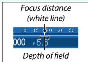
If both **AF DISTANCE INDICATOR** and **MF DISTANCE INDICATOR** are selected in the  **SCREEN SET-UP > DISP. CUSTOM SETTING** list, depth of field can also be previewed using the depth-of-field indicator in the standard display. Use the **DISP/BACK** button to display standard indicators.
