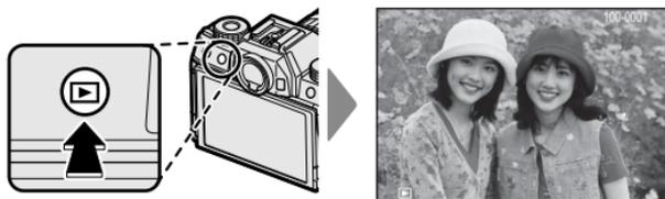
Additional pictures can be viewed by pressing the selector left or right or rotating the main command dial. Press the selector or rotate the dial right to view pictures in the order recorded, left to view pictures in reverse order. Keep the selector pressed to scroll rapidly to the desired frame.
