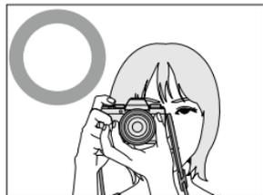
To prevent pictures that are out of focus or too dark (underexposed), keep your fingers and other objects away from the lens, flash, and AF-assist illuminator.
