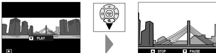
Press the selector down to start playback and press again to pause. Press the selector left or right to choose the pan direction while playback is in progress or to scroll the panorama manually while playback is paused; vertical panoramas will scroll vertically, horizontal panoramas horizontally. To exit to full-frame playback, press the selector up. To view other images, exit to full-frame playback and press the selector left or right.
