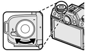
At shipment, the dial is assigned the **DEFAULT** role. At this setting, the function performed by the dial varies with the position of the mode dial.
