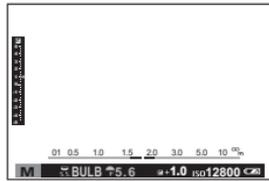
The shutter will remain open for up to 60 minutes, or for 1 second when the electronic shutter is used.
