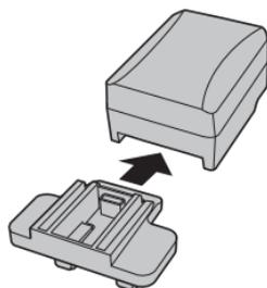
**!** The supplied plug adapter is for use exclusively with the AC-5VG AC power adapter. Do not use it with other devices.
