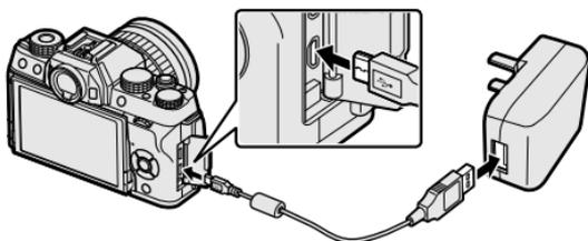
**!** Connect the cable to the camera's Micro USB (Micro-B) connector. Be sure the connectors are in the correct orientation and then insert them fully.
