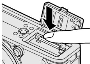
**!** Press the center of the card when ejecting it.
