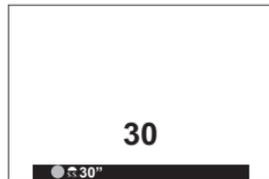
A count-down timer will be displayed while the exposure is in progress.
