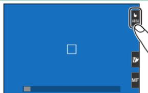
The touch screen mode indicator is not displayed and touch controls cannot be used when **OFF** is selected for **TOUCH SCREEN SETTING > TOUCH SCREEN ON/OFF** in the setup menu.
