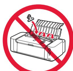
Do not allow objects to fall inside the printer. These could cause malfunction.
