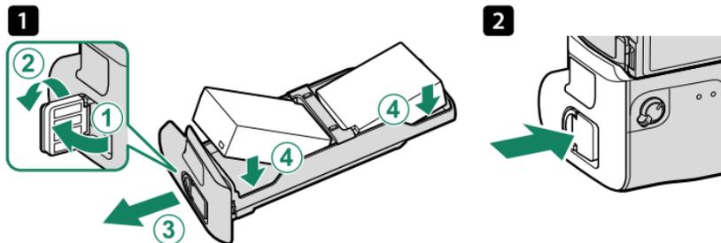
The batteries can be removed as shown.
