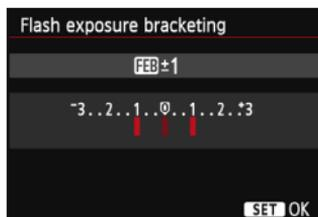
While the flash output is changed automatically, three shots are taken. For details, refer to the instruction manual of a Speedlite compatible with flash exposure bracketing.
